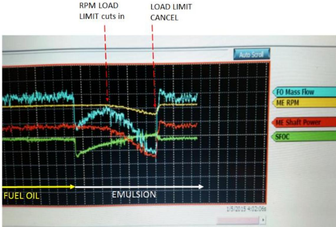
Fig 6: Effects on main engine when RPM-Load limit is exceeded.
